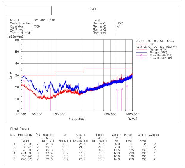
Note 1) Receiving antenna polarization : Horizontal, Vertical Test Distance : 10 m, Antenna Height : 1 to 4 meters
