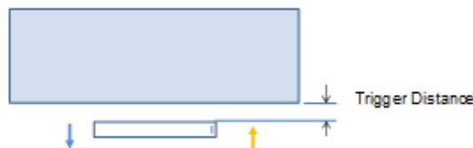
Proximity Sensor Trigger Distance Assessment KDB 616217 §6.2, Front
