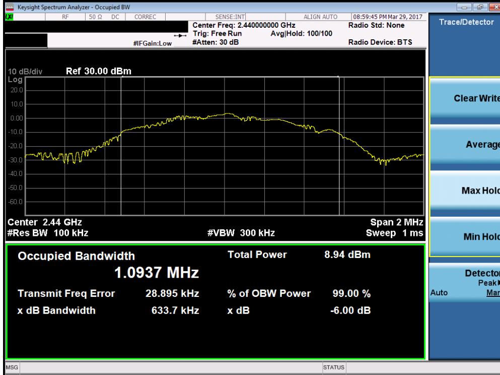
Plot 7-2. 6dB Bandwidth Plot (Bluetooth (LE) – Ch. 19)
