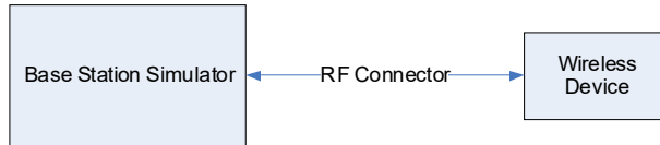
Figure 9-2 Power Measurement Setup
