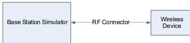
Figure 9-3 Power Measurement Setup
