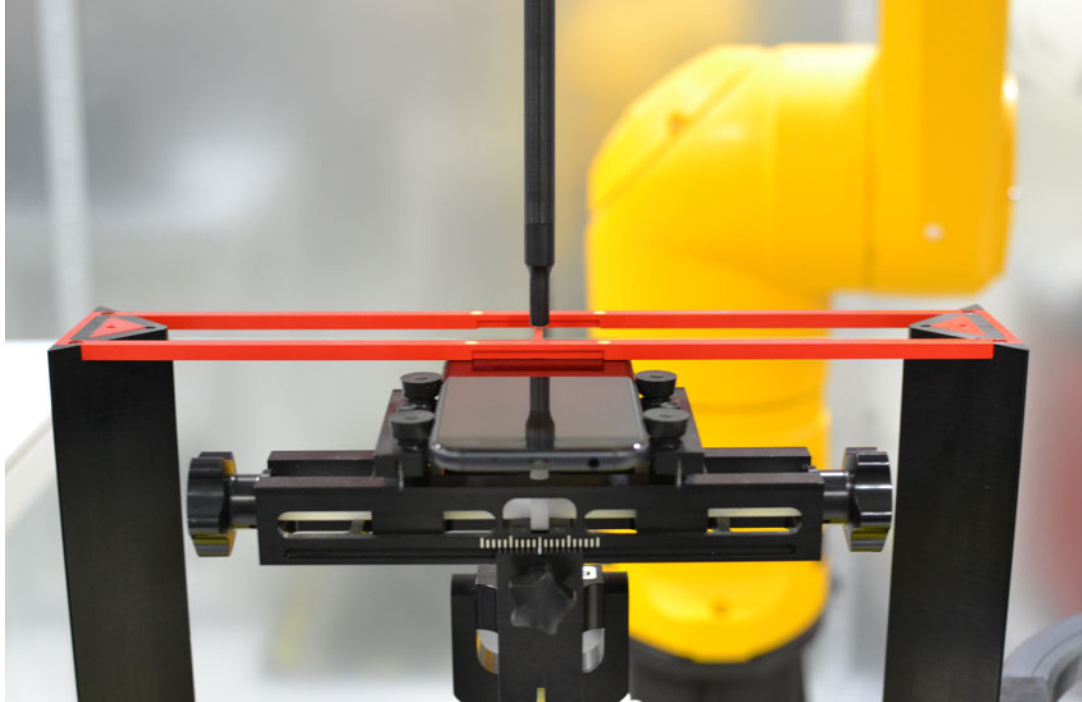
Figure 18-1 Ear Reference Point HAC Phantom Alignment
