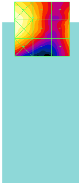
Figure 11-1 Sample E-field Scan Overlay (See Test Setup Photographs for actual WD overlay)
