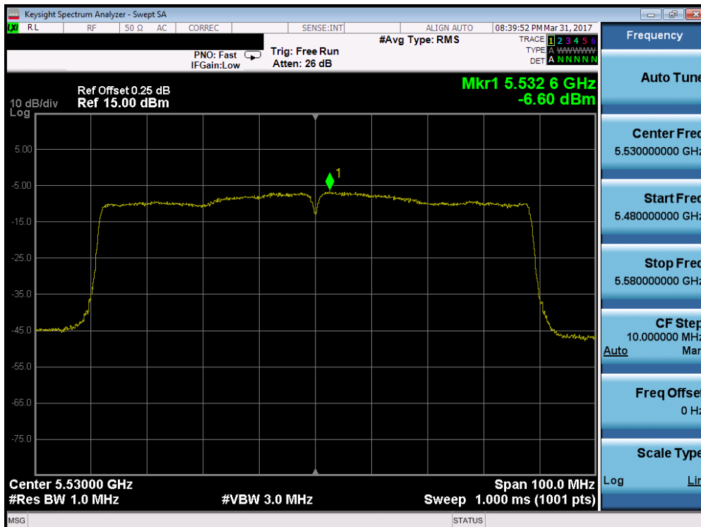
Plot 7-67. Power Spectral Density Plot (80MHz BW 802.11ac (UNII Band 2C) – Ch. 106)
