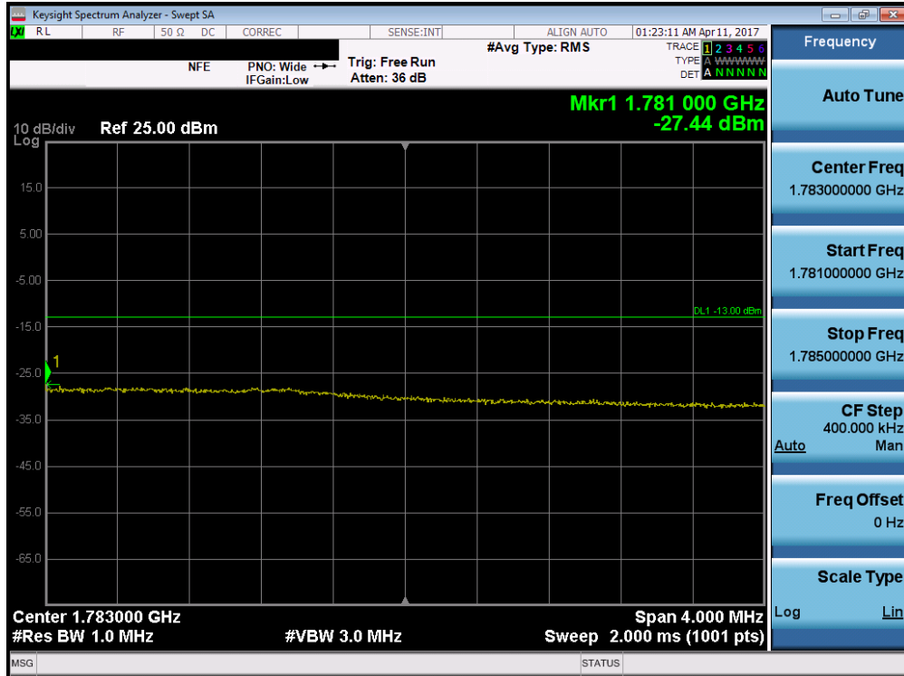
Plot 7-131. Upper Extended Band Edge Plot (Band 4/66 – 15.0MHz QPSK – RB Size 75)
