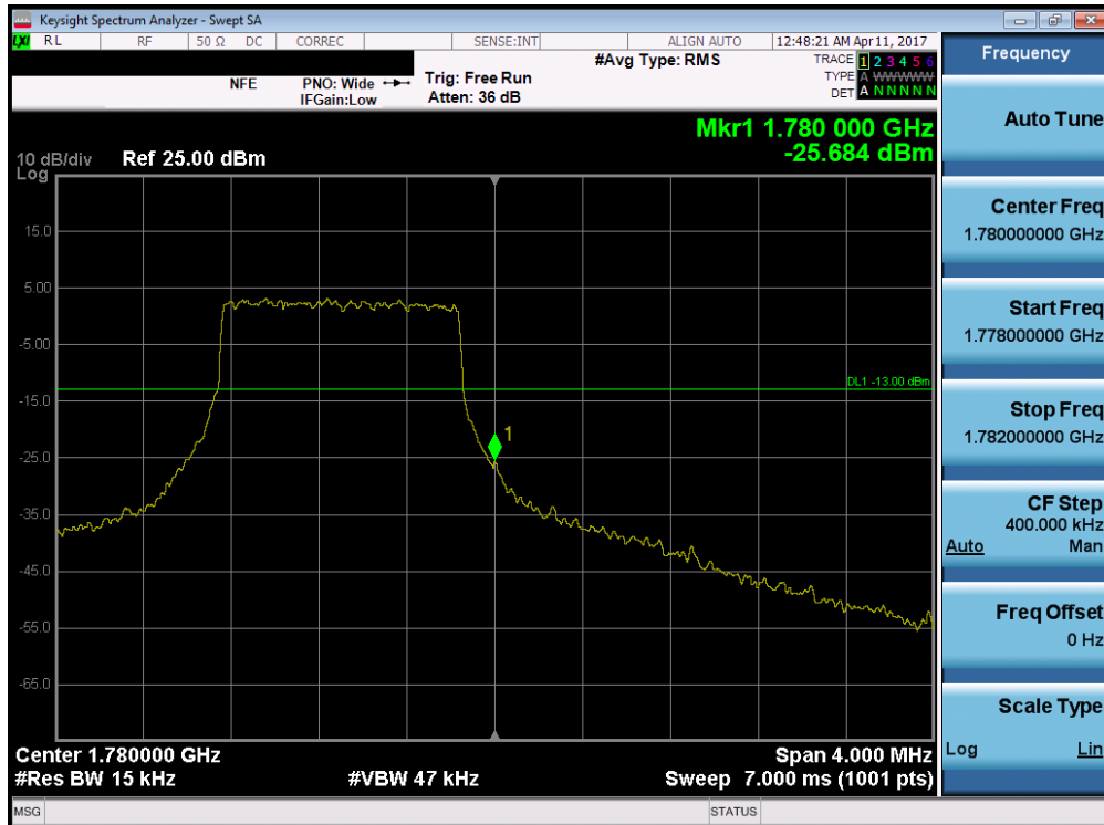
Plot 7-114. Upper Band Edge Plot (Band 4/66 – 1.4MHz QPSK – RB Size 6)
