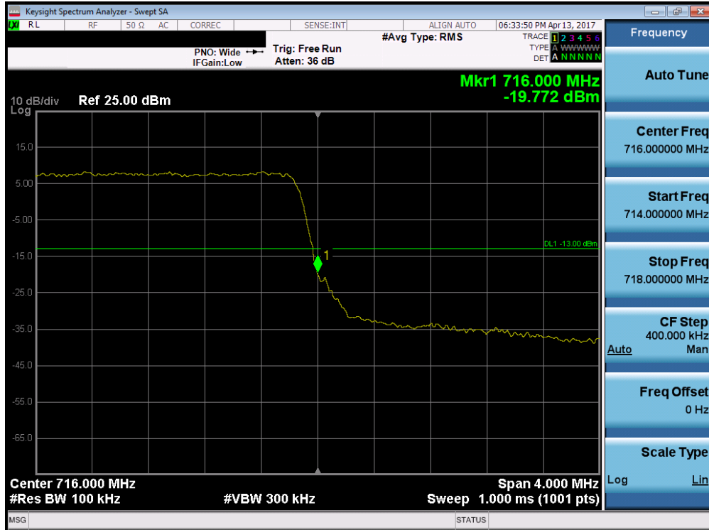
Plot 7-97. Upper Band Edge Plot (Band 12 – 3.0MHz QPSK – RB Size 15)
