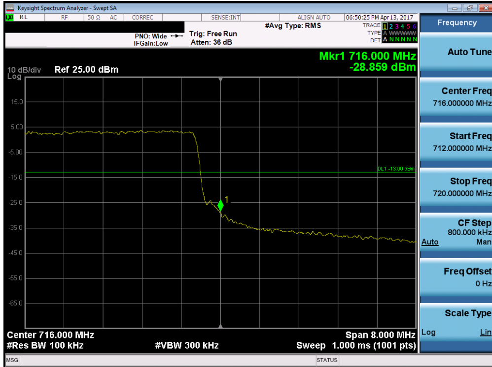
Plot 7-101. Upper Band Edge Plot (Band 12/17 – 10.0MHz QPSK – RB Size 50)
