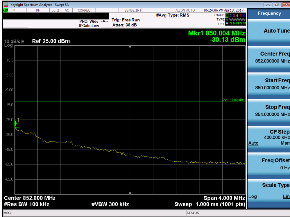
Plot 7-105. Upper Extended Band Edge Plot (Band 5 – 1.4MHz QPSK – RB Size 6)
