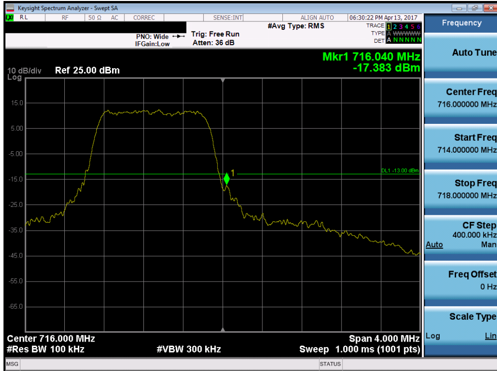
Plot 7-95. Upper Band Edge Plot (Band 12 – 1.4MHz QPSK – RB Size 6)
