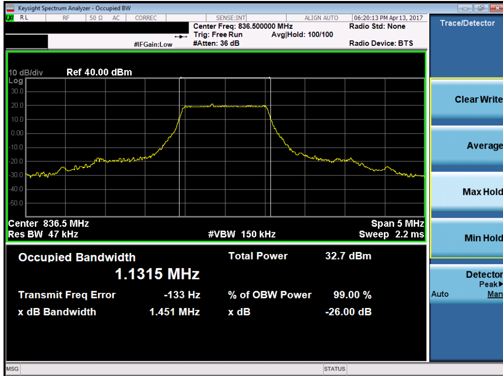
Plot 7-9. Occupied Bandwidth Plot (Band 5 – 1.4MHz QPSK – RB Size 6)
