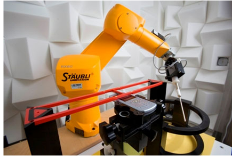
Figure 4-3 SPEAG Robotic System
