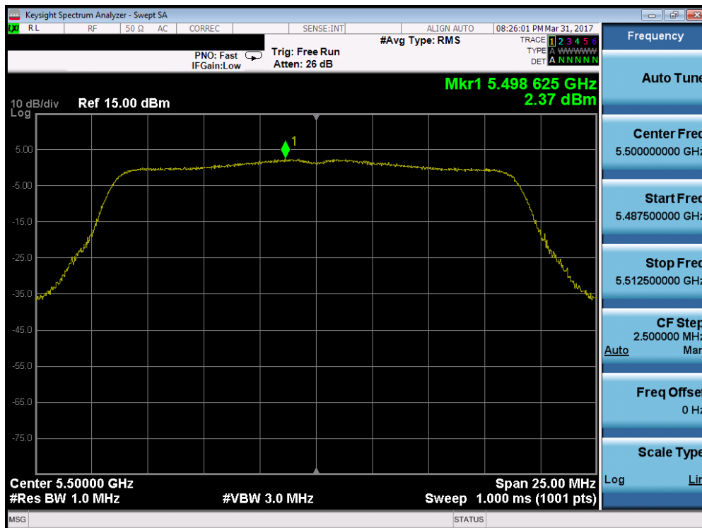
Plot 7-61. Power Spectral Density Plot (20MHz BW 802.11n (UNII Band 2C) – Ch. 100)
