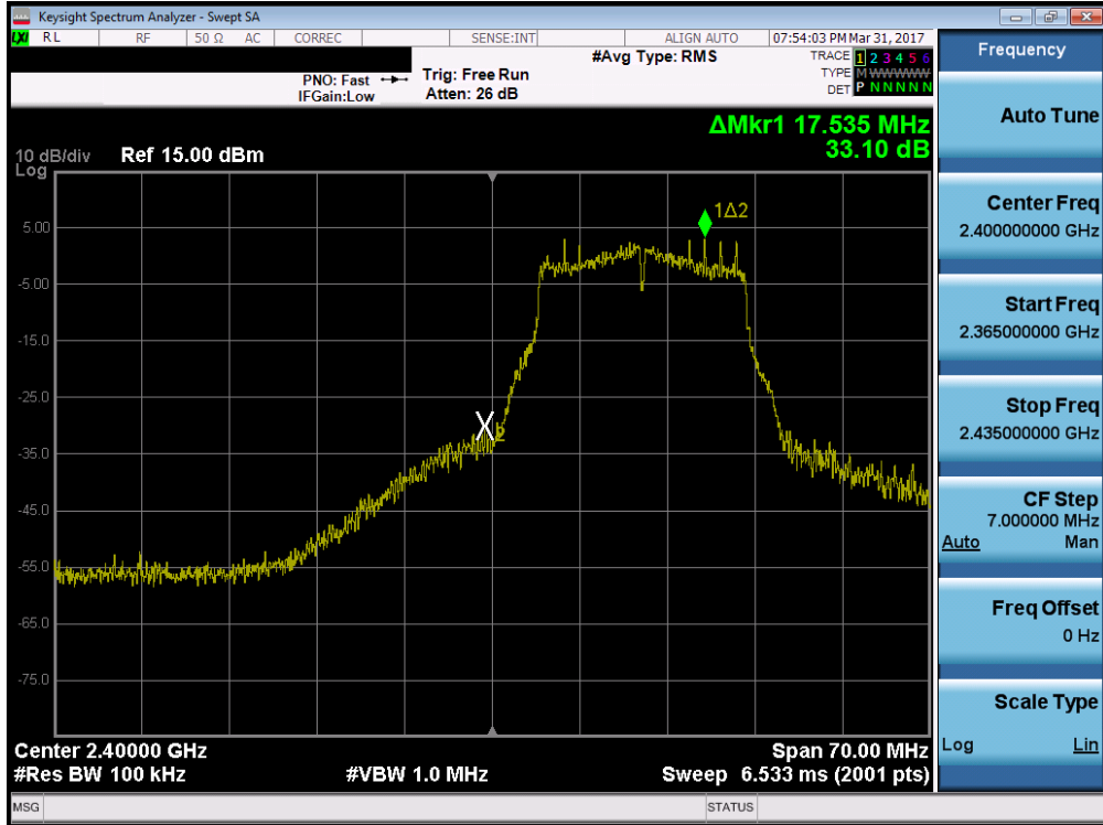
Plot 7-21. Band Edge Plot (802.11g– Ch. 1)
