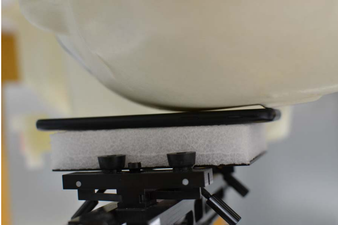
SAR Test Setup Photo 3 – Left Cheek
