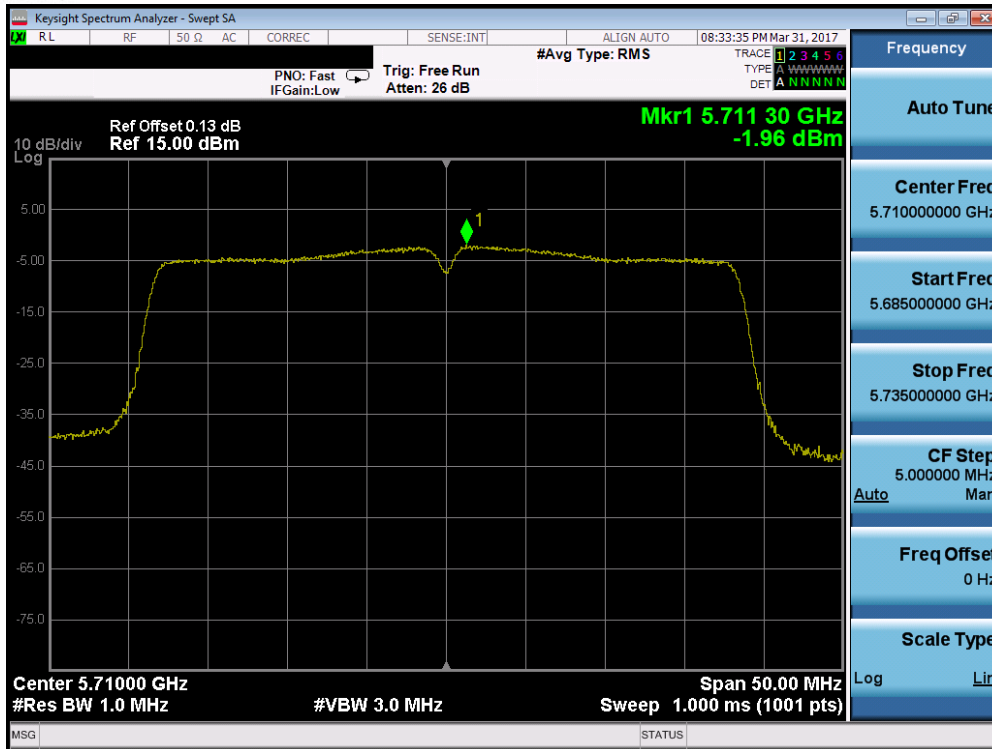
Plot 7-66. Power Spectral Density Plot (40MHz BW 802.11n (UNII Band 2C) – Ch. 142)
