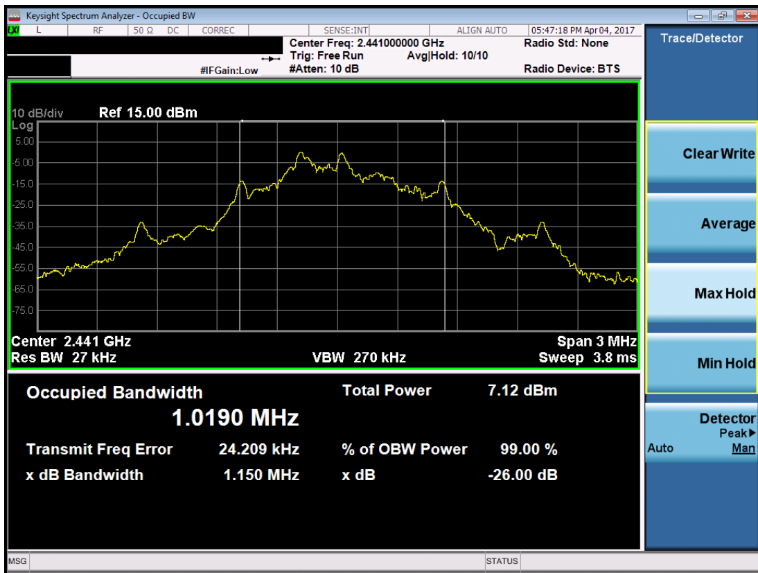
Plot 7-1. Occupied Bandwidth Plot (ANT+ – Ch. 39)
