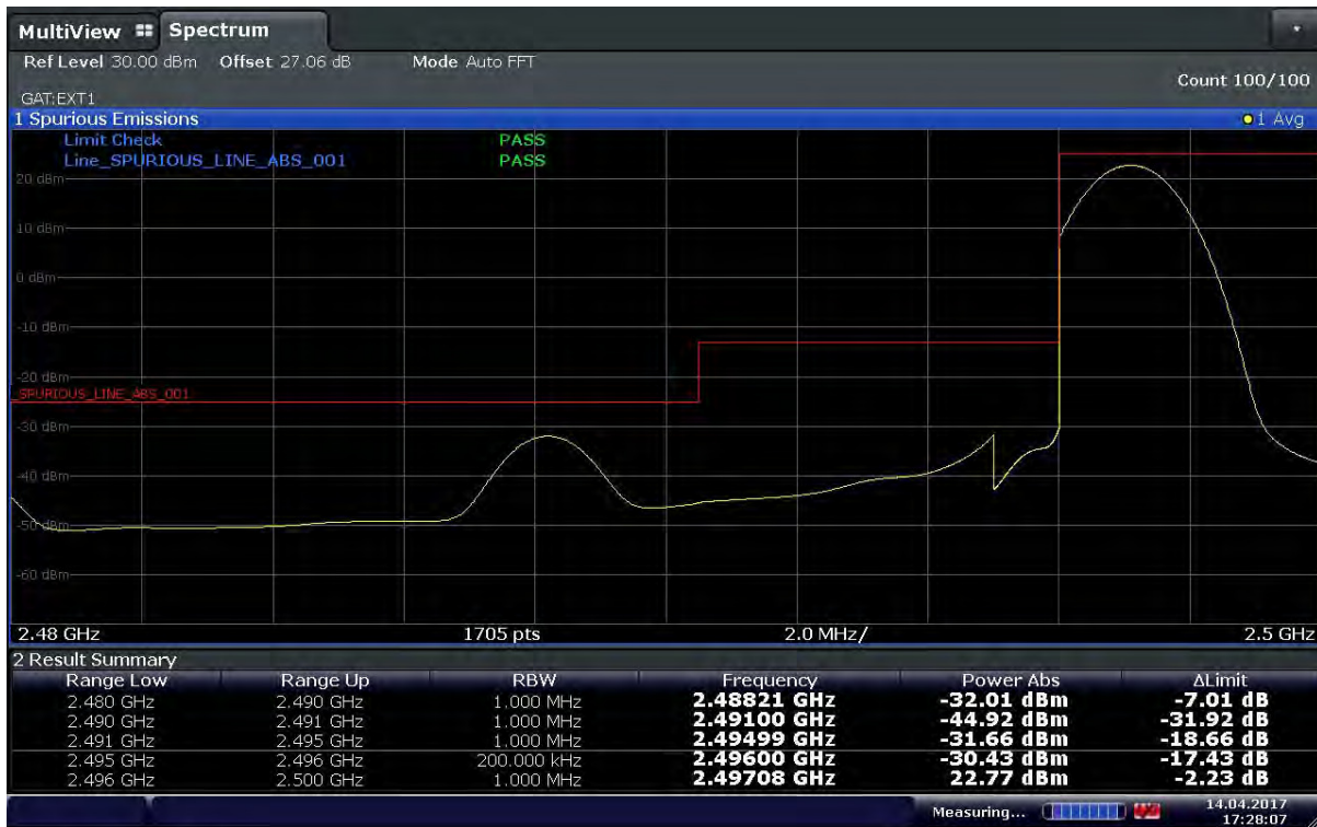
Plot 6-75. Lower Band Edge Plot (Band41 – 20MHz – QPSK – RB Size 1 – RB Offset 0 – Ch.39750)
