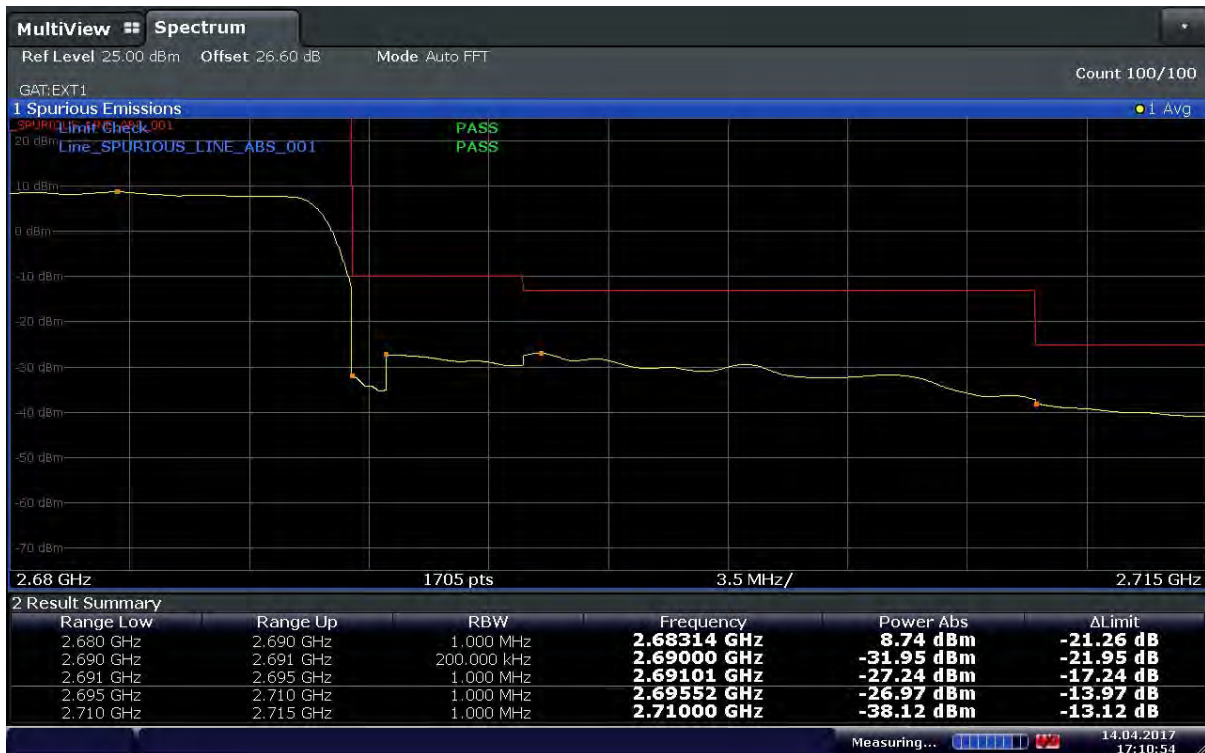
Plot 6-74. Upper Band Edge Plot (Band41 – 20MHz – QPSK – RB Size 100 – Ch.41490)
