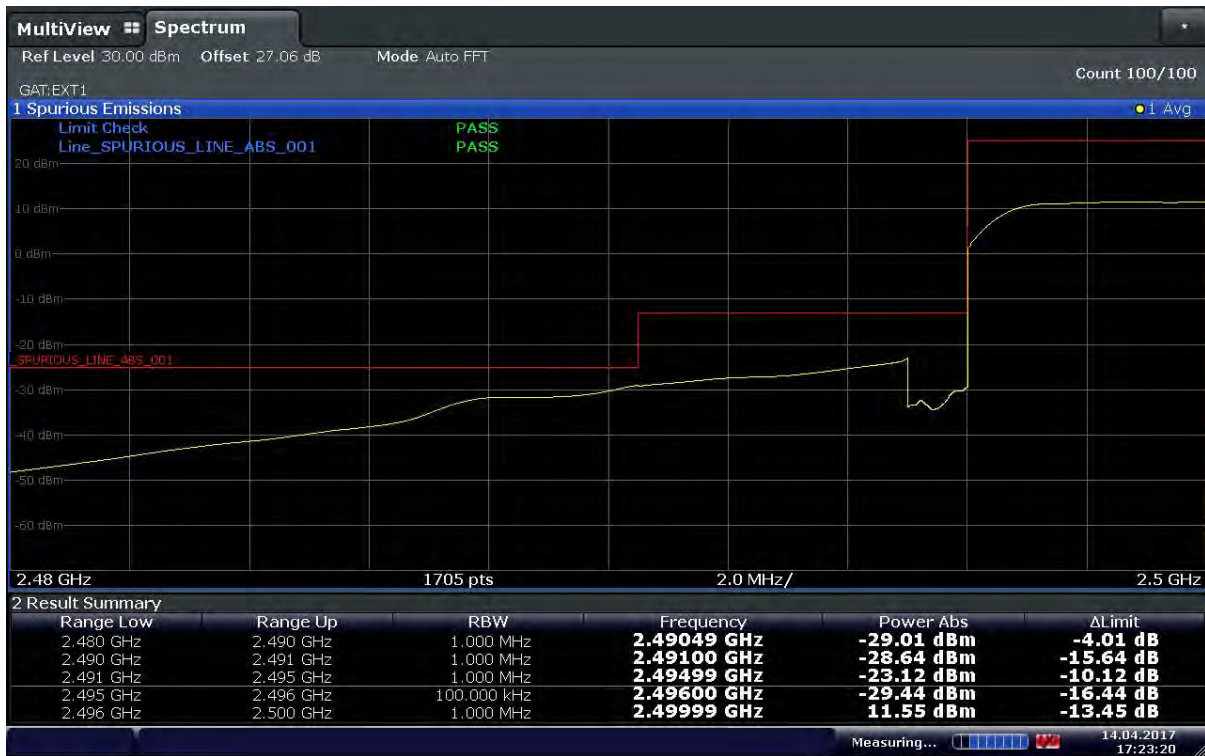
Plot 6-69. Lower Band Edge Plot (Band41 – 10MHz – QPSK – RB Size 50 – Ch.39700)
