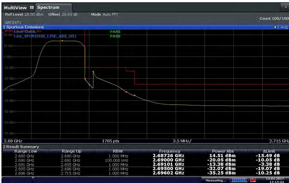
Plot 6-68. Upper Band Edge Plot (Band41 – 5MHz – QPSK – RB Size 25 – Ch.41565)
