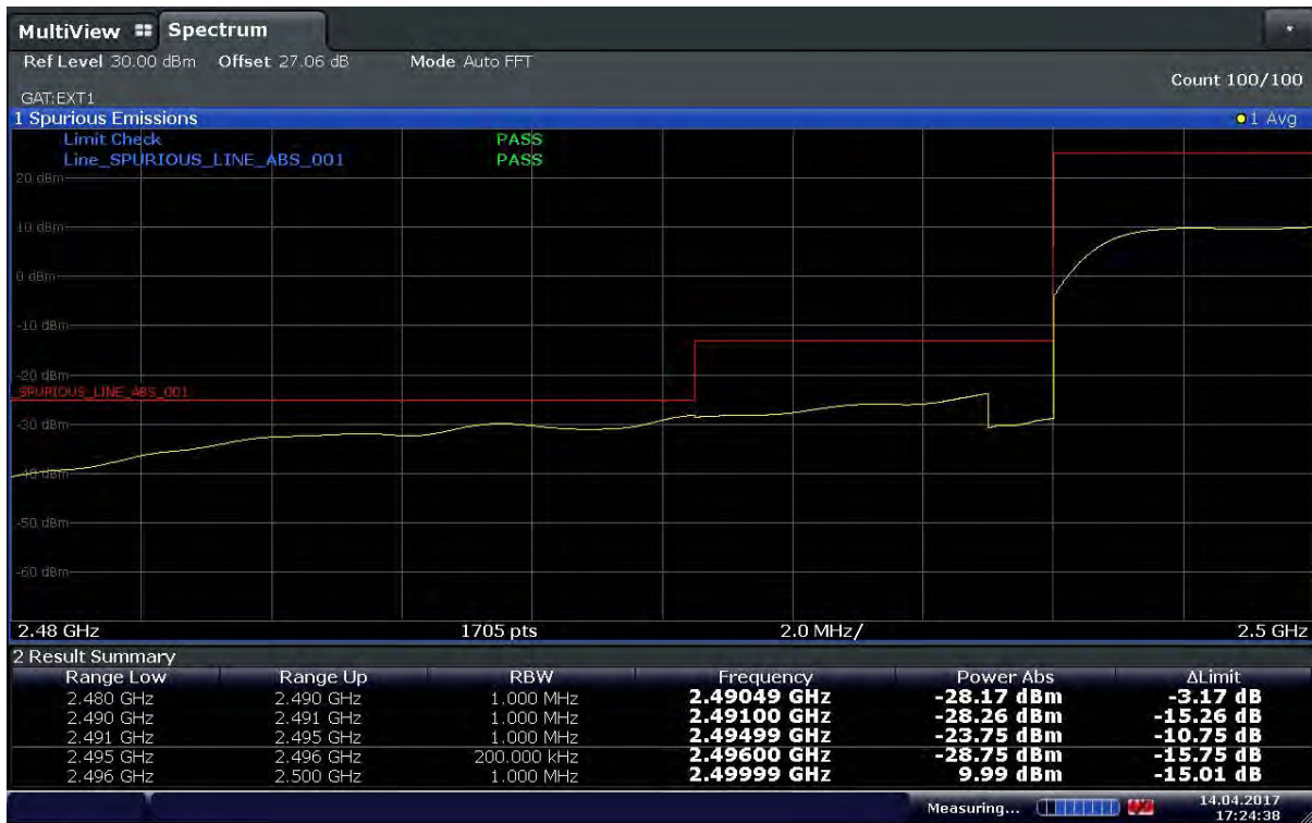
Plot 6-71. Lower Band Edge Plot (Band41 – 15MHz – QPSK – RB Size 75 – Ch.39725)
