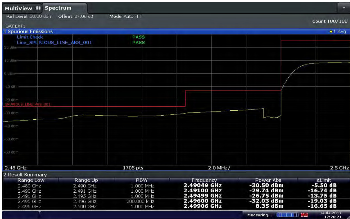
Plot 6-73. Lower Band Edge Plot (Band41 – 20MHz – QPSK – RB Size 100 – Ch.39750)
