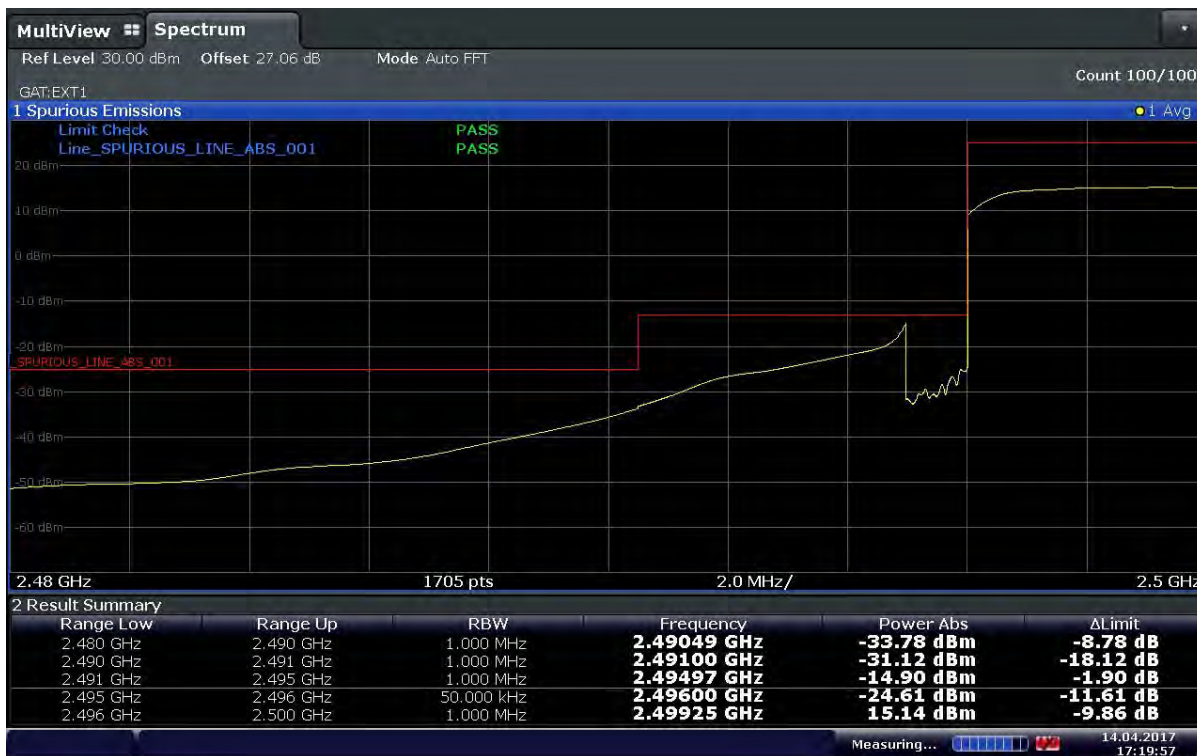
Plot 6-67. Lower Band Edge Plot (Band41 – 5MHz – QPSK – RB Size 25 – Ch.39675)
