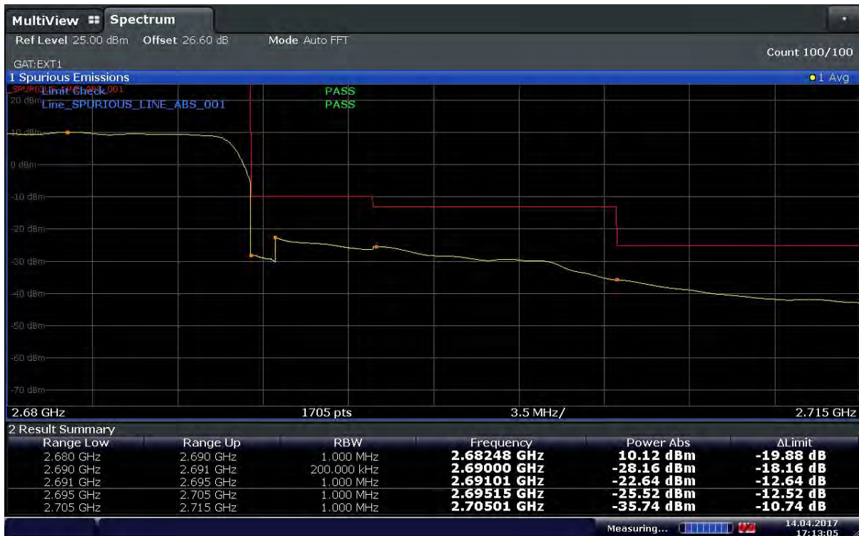
Plot 6-72. Upper Band Edge Plot (Band41 – 15MHz – QPSK – RB Size 75 – Ch.41515)
