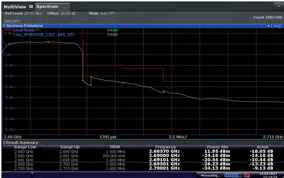
Plot 6-70. Upper Band Edge Plot (Band41 – 10MHz – QPSK – RB Size 50 – Ch.41540)
