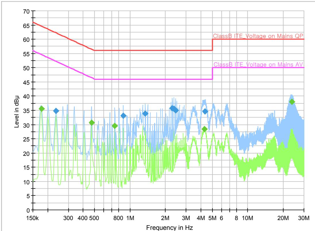
Note 1) Two graphs measured for both Live(L1) and Neutral(N) of the LISN are combined into one graph.
