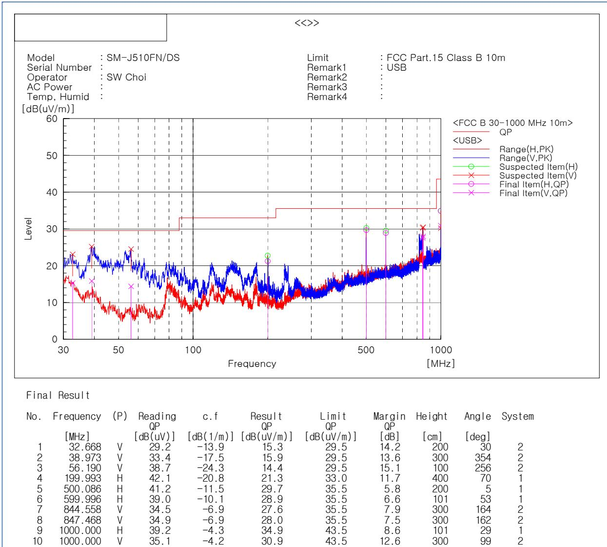
Note) Receiving antenna polarization : Horizontal, Vertical
