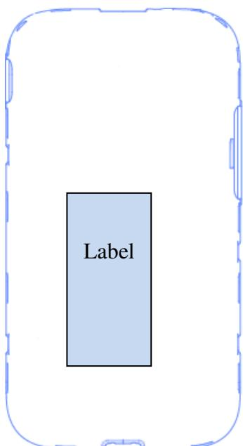
Phone: Label is placed inside of the battery compartment.
