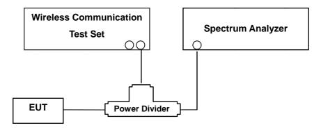
(Configuration of conducted Emission measurement)
