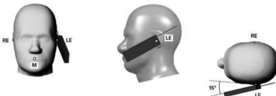
Figure 6.5. Tilt 15^\circ position of the wireless device
