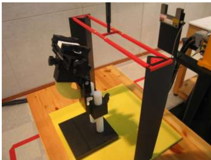
Figure 2. HAC Phantom & Device Holder
