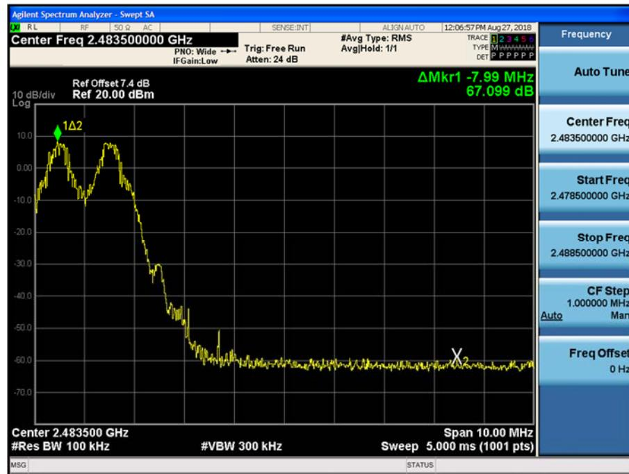
Test Plots with hopping (8DPSK)
