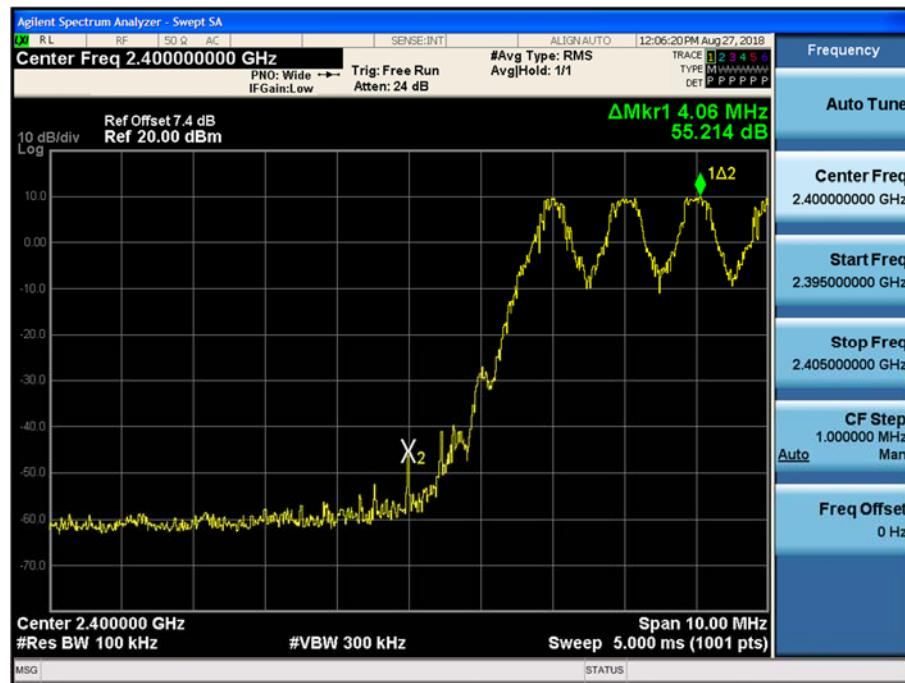
Test Plots with hopping (GFSK)
