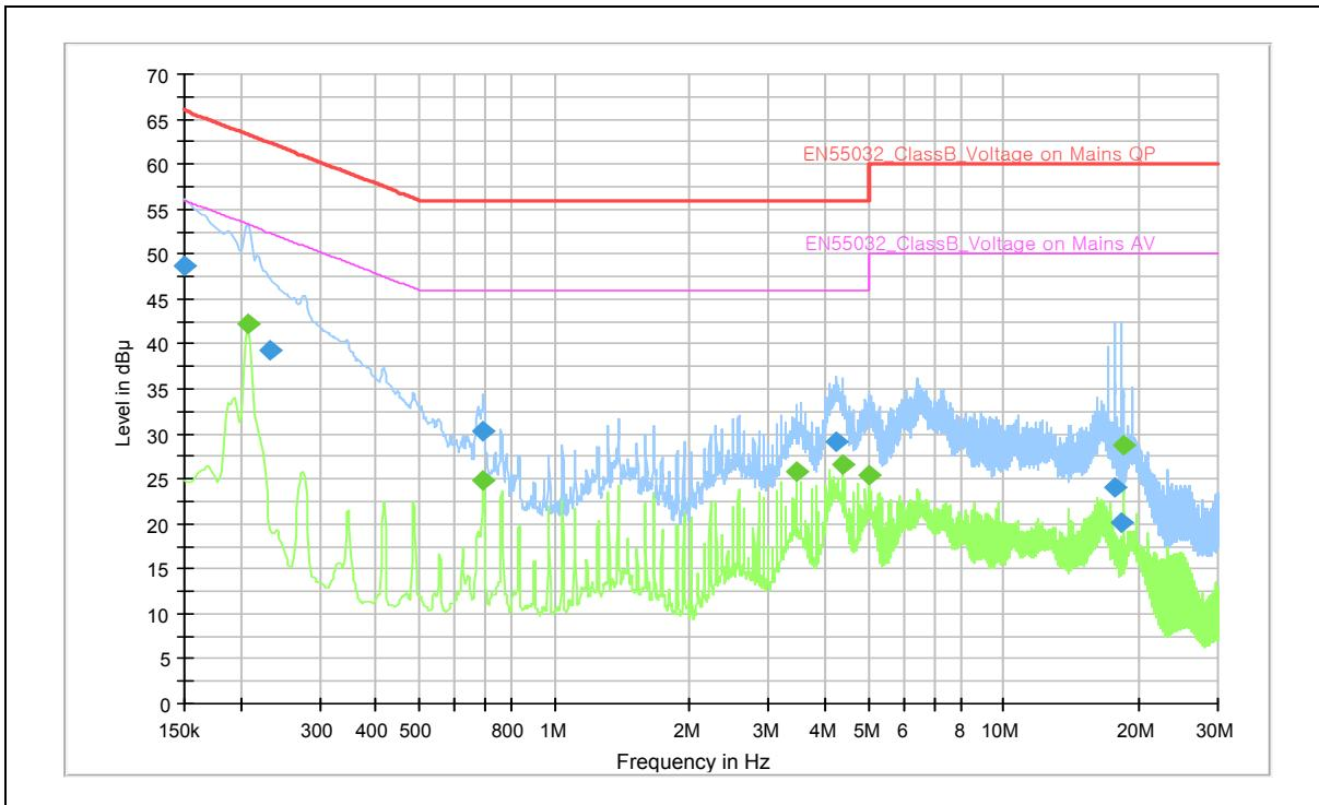
Note 1) Two graphs measured for both Live(L1) and Neutral(N) of the LISN are combined into one graph.
