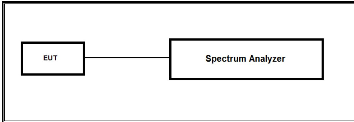
**SETUP DIAGRAM FOR TESTS (RADIATED TEST SETUP)**
