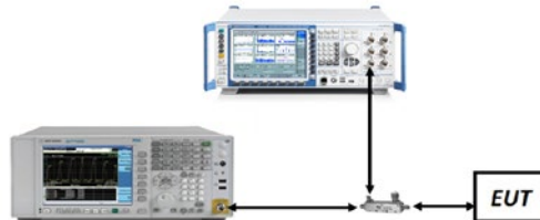
Figure 7-2. Test Instrument & Measurement Setup
