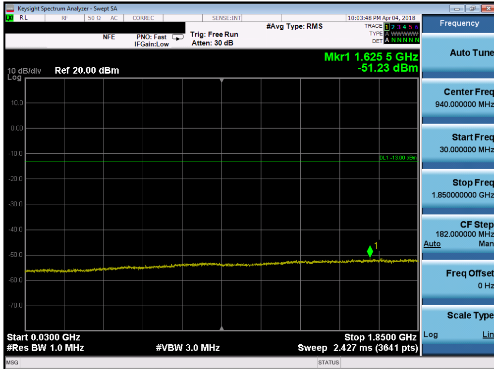
Plot 7-39. Conducted Spurious Plot (PCS CDMA Mode - Mid Channel)
