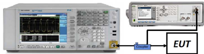
Figure 7-6. Test Instrument & Measurement Setup
