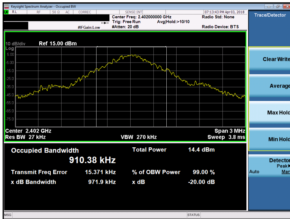
Plot 7-1. 20dB Bandwidth Plot (Bluetooth, 1Mbps – Ch. 0)
