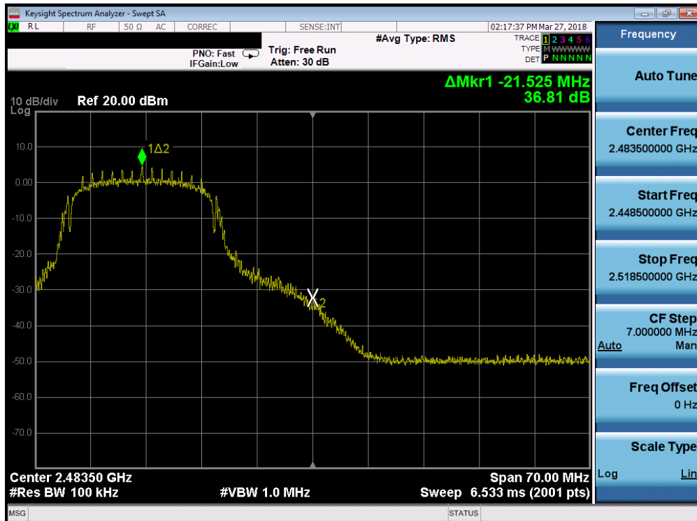
Plot 7-24. Band Edge Plot (802.11n (2.4GHz) – Ch. 11)
