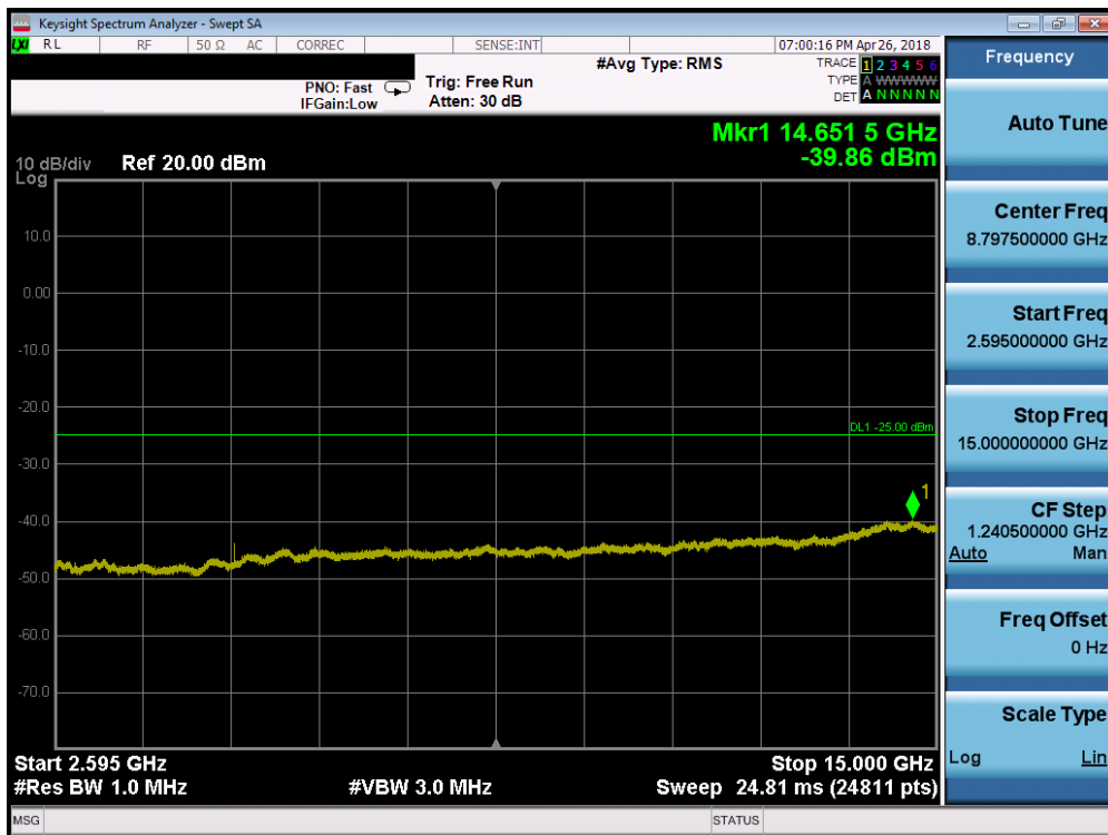
Plot 7-82. Conducted Spurious Plot (Band 7 - 10.0MHz QPSK - RB Size 1, RB Offset 0 - High Channel)
