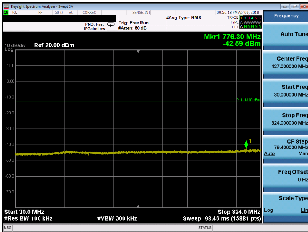
Plot 7-51. Conducted Spurious Plot (Band 5 - 10.0MHz QPSK - RB Size 1, RB Offset 0 - Mid Channel)
