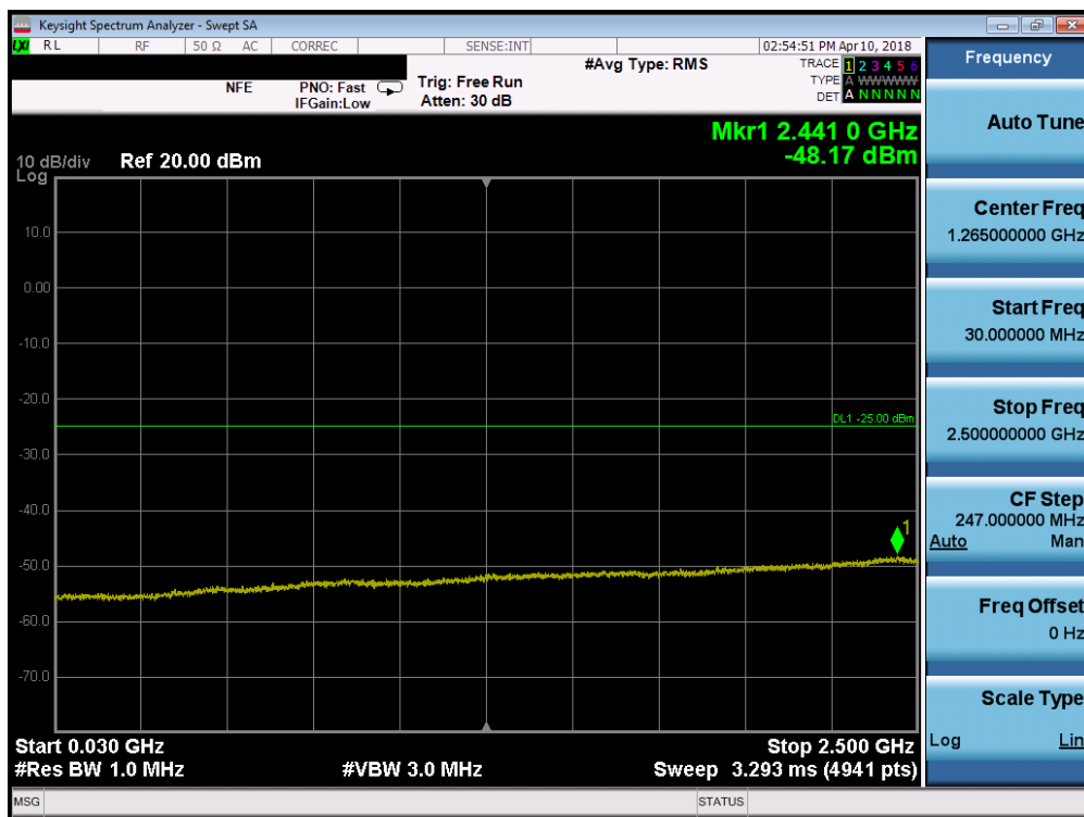
Plot 7-78. Conducted Spurious Plot (Band 7 - 10.0MHz QPSK - RB Size 1, RB Offset 0 - Mid Channel)
