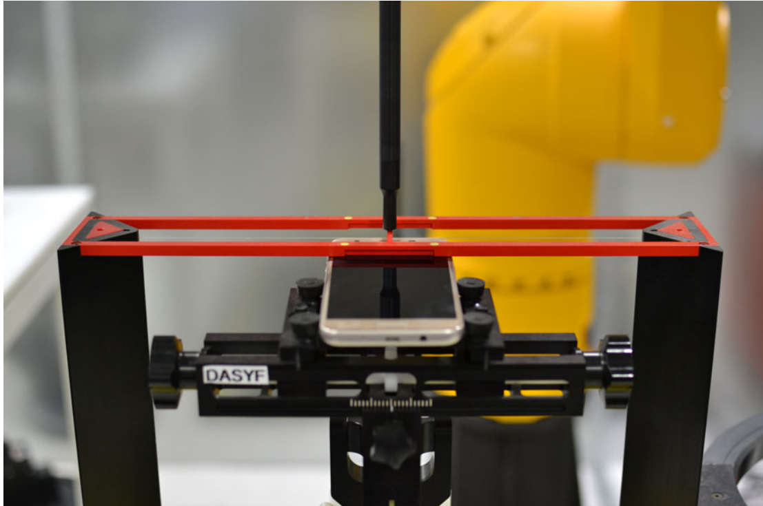
Figure 17-1 Ear Reference Point HAC Phantom Alignment
