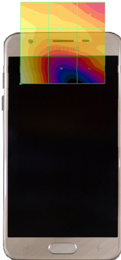
Figure 17-4 E-Field WD Scan overlay
