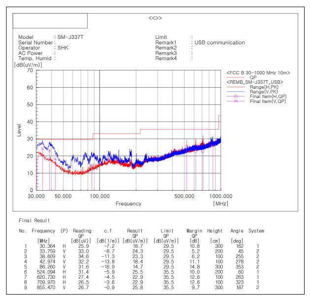
Note) Receiving antenna polarization: Horizontal, Vertical
