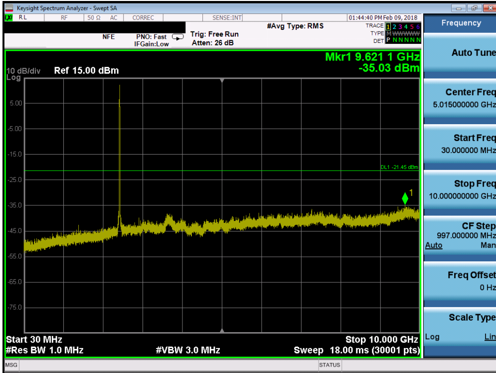
Plot 7-27. Conducted Spurious Plot (802.11b – Ch. 6)
