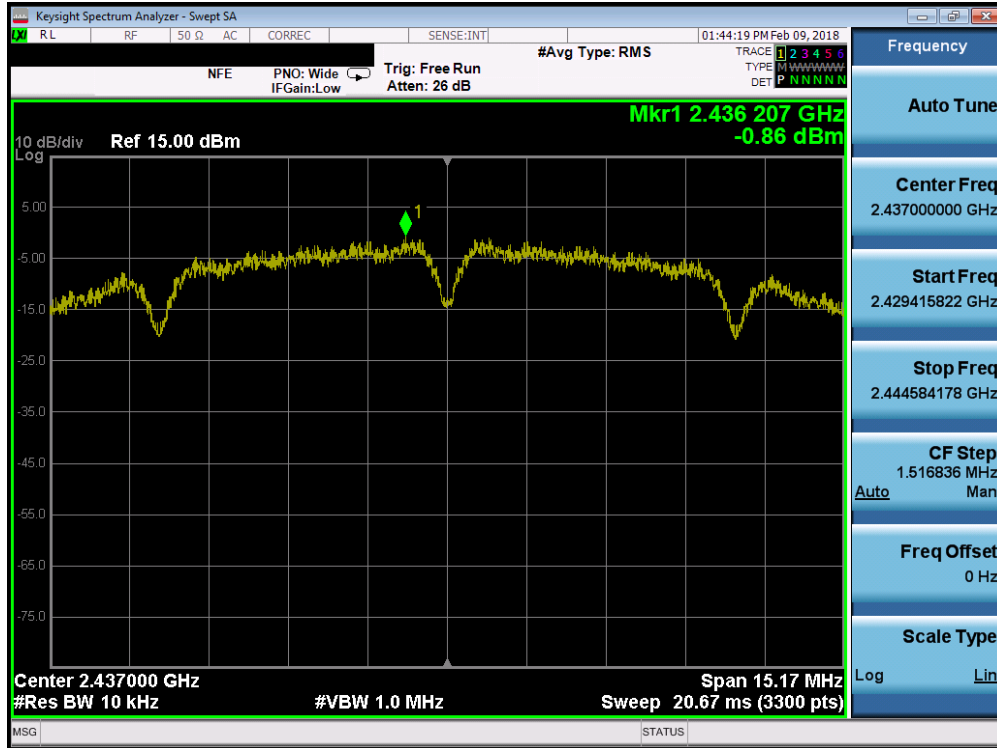
Plot 7-11. Power Spectral Density Plot (802.11b – Ch. 6)
