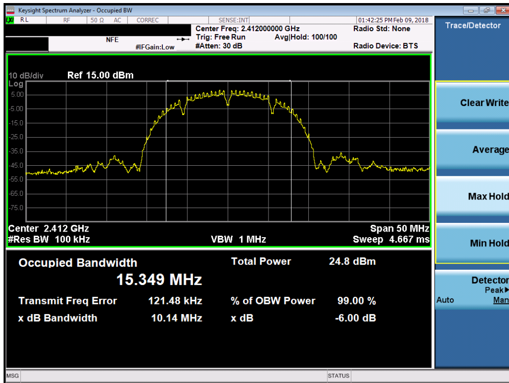
Plot 7-1. 6dB Bandwidth Plot (802.11b – Ch. 1)
