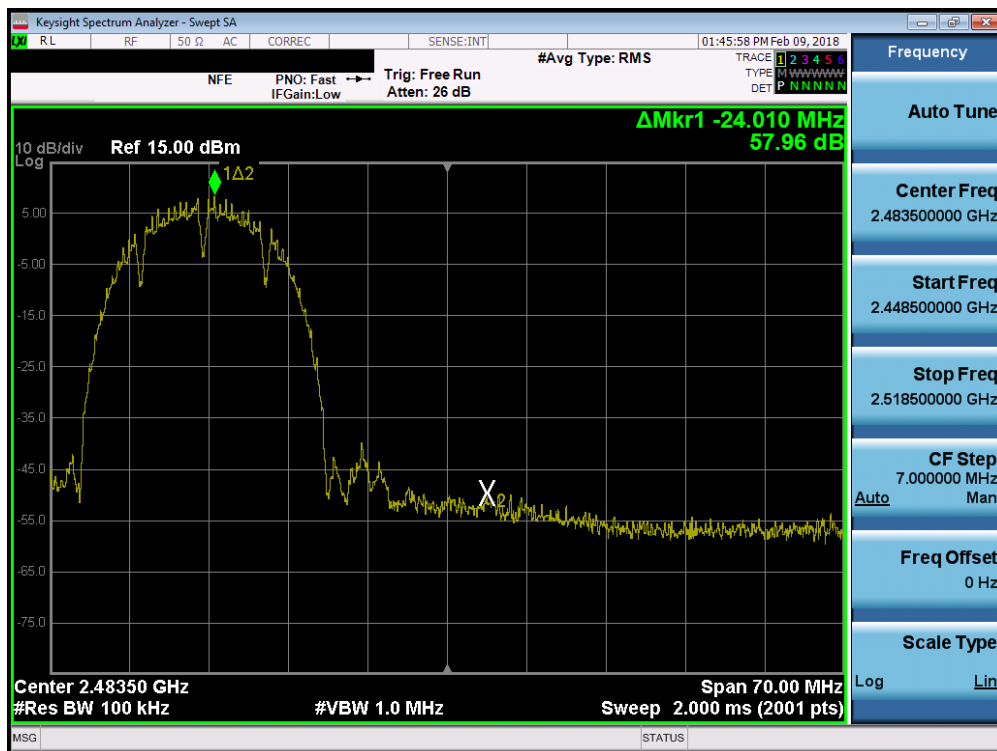
Plot 7-20. Band Edge Plot (802.11b – Ch. 11)
