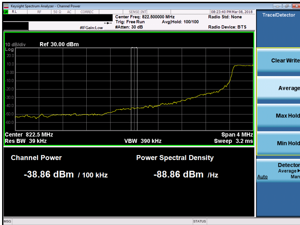
Plot 7-129. Lower Extended Band Edge Plot (Band 5 - 1.4MHz QPSK - Full RB Configuration)
