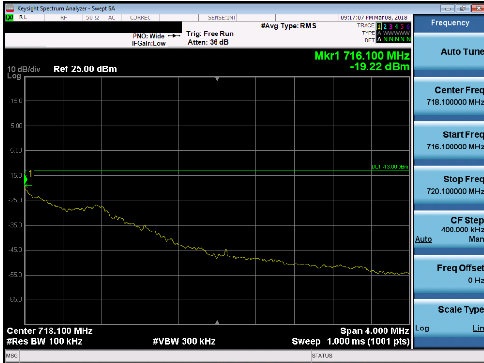
Plot 7-121. Upper Extended Band Edge Plot (Band 12 - 1.4MHz QPSK - Full RB Configuration)
