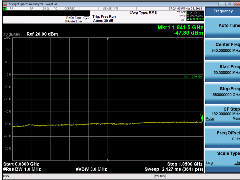
Plot 7-99. Conducted Spurious Plot (Band 2 - 10.0MHz QPSK - RB Size 1, RB Offset 0 - High Channel)
