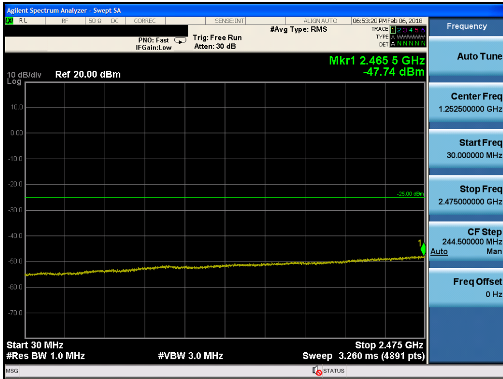
Plot 7-102. Conducted Spurious Plot (Band 7 - 10.0MHz QPSK - RB Size 1, RB Offset 0 - Low Channel)
