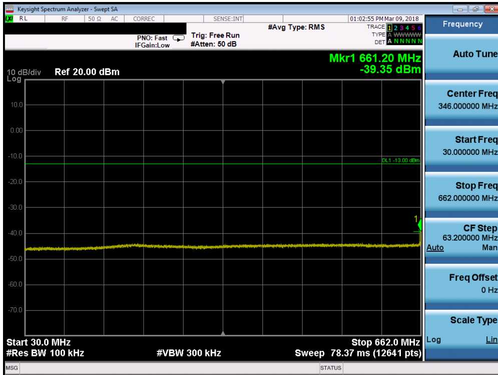
Plot 7-57. Conducted Spurious Plot (Band 71 - 5.0MHz QPSK - RB Size 1, RB Offset 0 - Low Channel)
