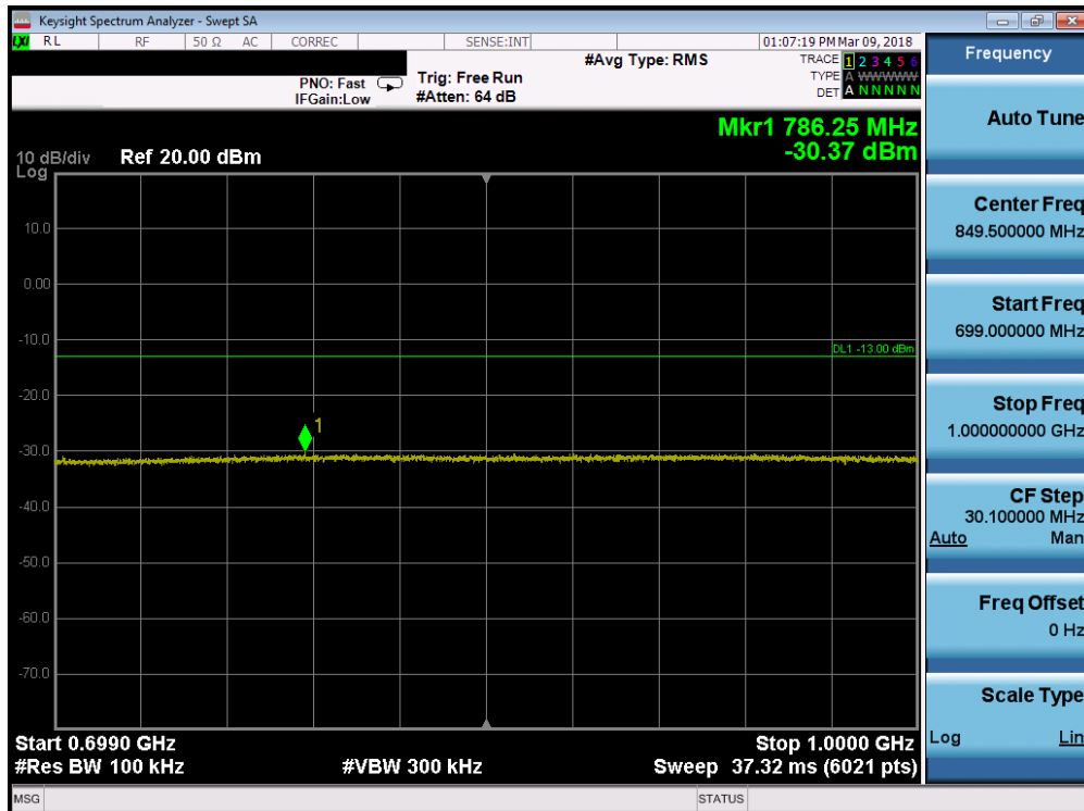
Plot 7-64. Conducted Spurious Plot (Band 71 - 5.0MHz QPSK - RB Size 1, RB Offset 0 - High Channel)
