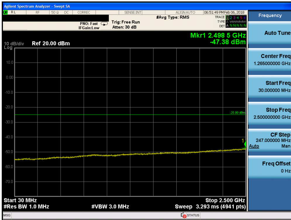
Plot 7-105. Conducted Spurious Plot (Band 7 - 10.0MHz QPSK - RB Size 1, RB Offset 0 - Mid Channel)
