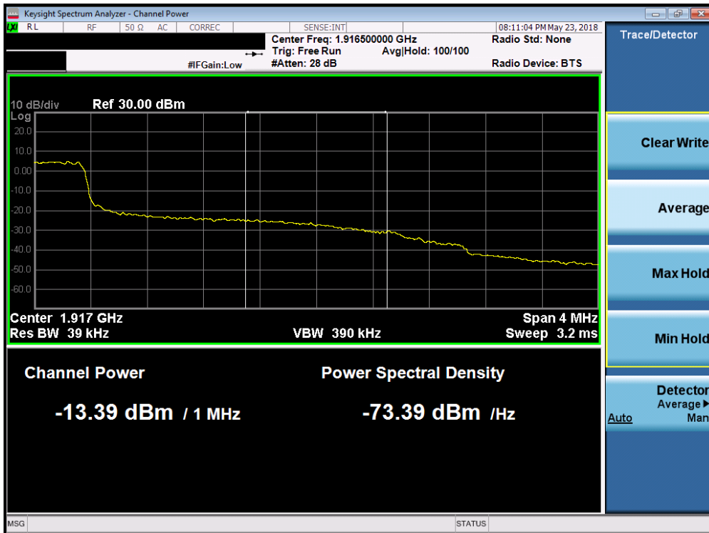
Plot 7-128. Upper Extended Band Edge Plot (Band 25 - 3.0MHz QPSK - Full RB Configuration)
