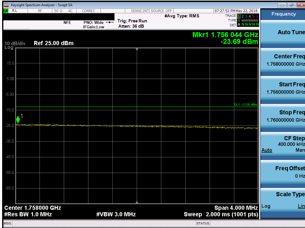
Plot 7-116. Upper Extended Band Edge Plot (Band 4 - 20.0MHz QPSK - Full RB Configuration)
