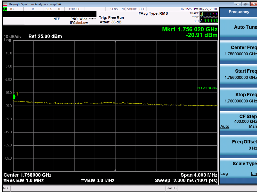
Plot 7-112. Upper Extended Band Edge Plot (Band 4 - 15.0MHz QPSK - Full RB Configuration)
