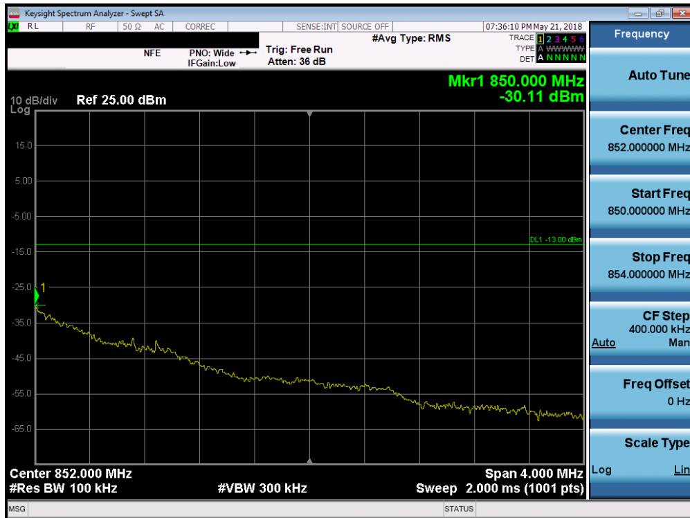
Plot 7-87. Upper Extended Band Edge Plot (Band 5 - 1.4MHz QPSK - Full RB Configuration)
