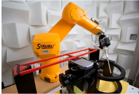
Figure 4-3 SPEAG Robotic System
