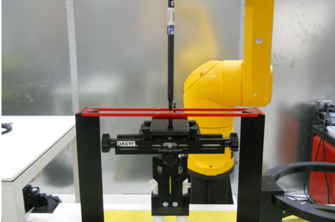
Figure 18-1 Ear Reference Point HAC Phantom Alignment
