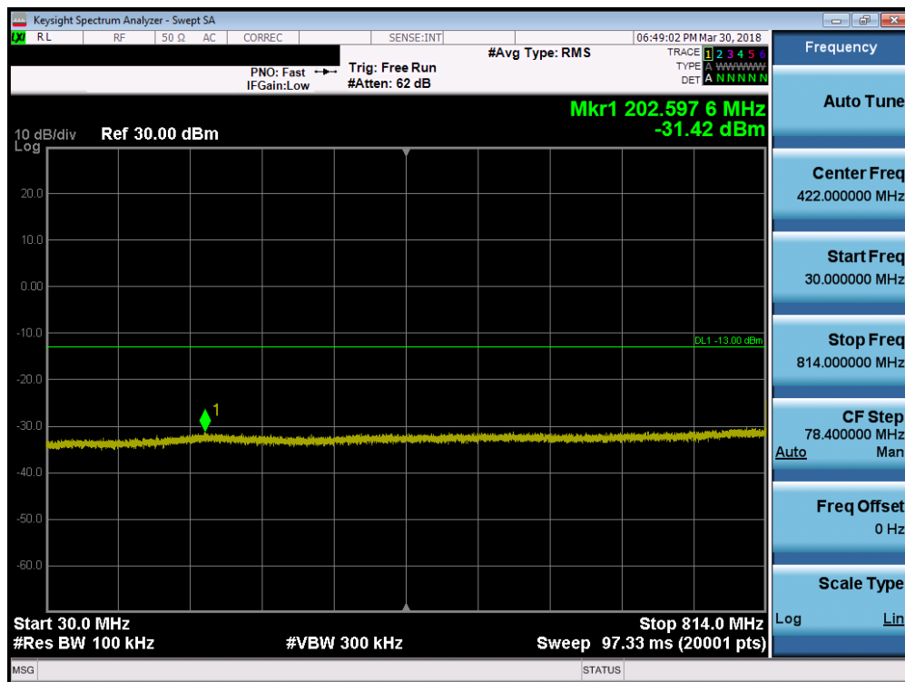
Plot 7-18. Conducted Spurious Plot ( LTE B26 - 15MHz QPSK – RB Size 1, RB Offset 0 – Mid Channel)
