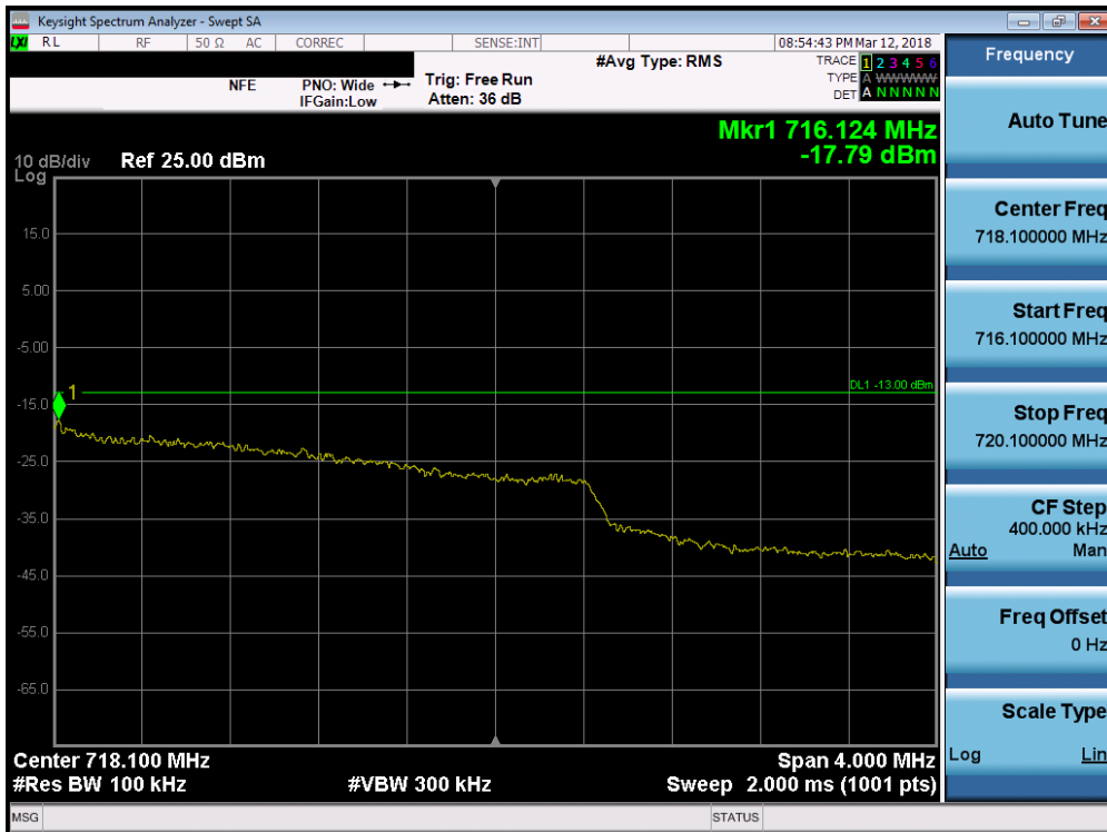
Plot 7-118. Upper Extended Band Edge Plot (Band 12 - 3.0MHz QPSK - Full RB Configuration)
