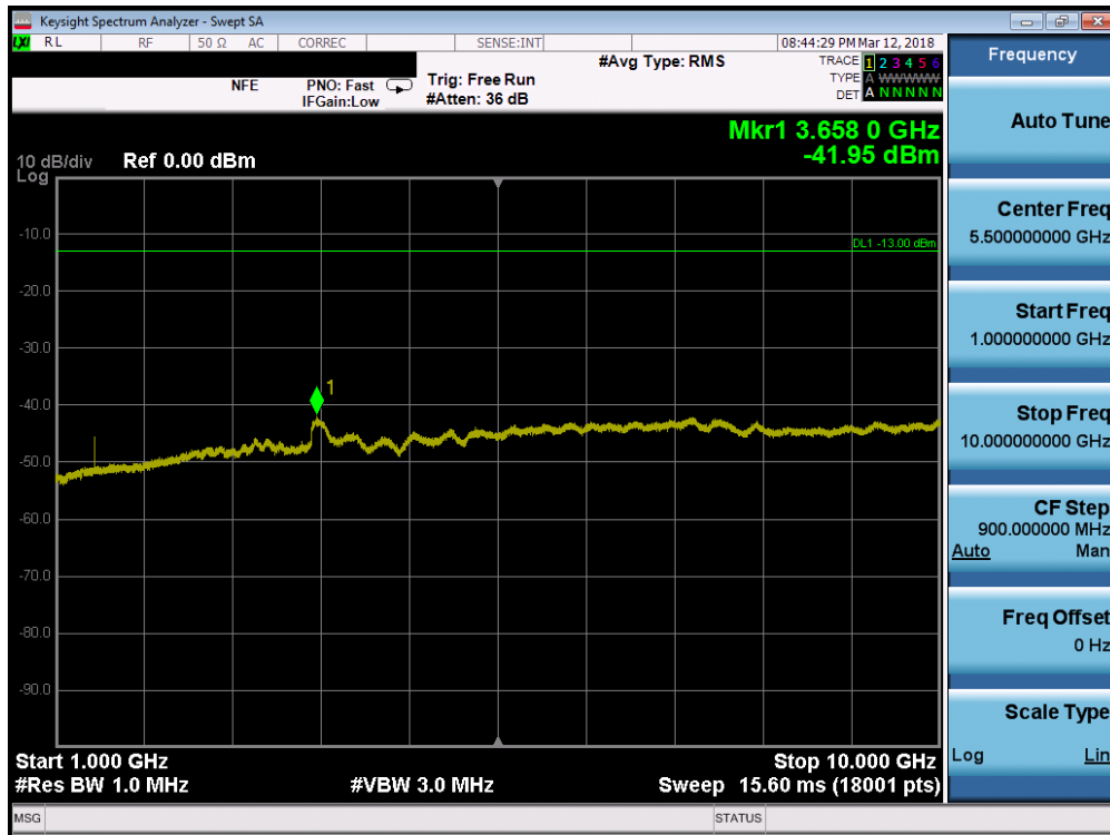
Plot 7-61. Conducted Spurious Plot (Band 12 - 10.0MHz QPSK - RB Size 1, RB Offset 0 - Low Channel)
