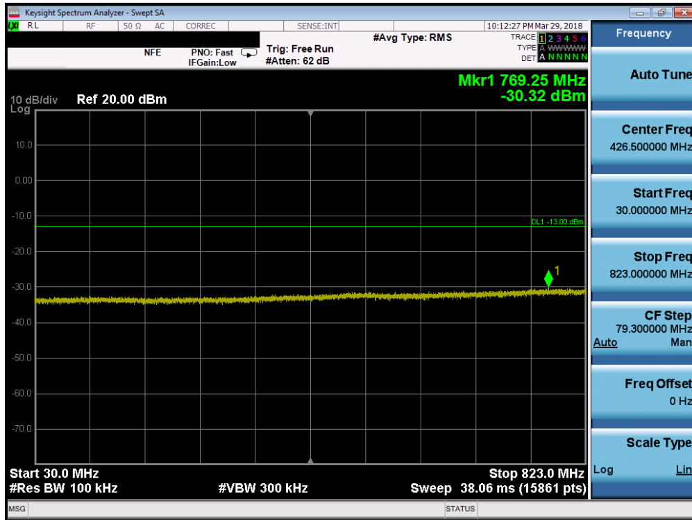
Plot 7-68. Conducted Spurious Plot (Band 26/5 - 10.0MHz QPSK - RB Size 1, RB Offset 0 - Low Channel)
