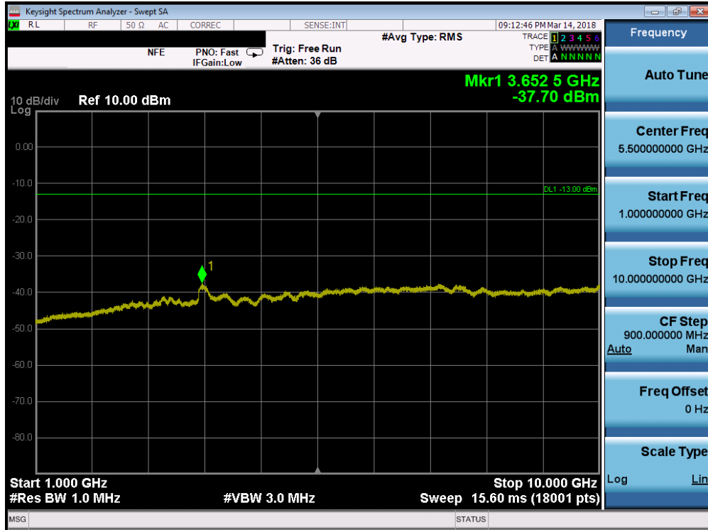
Plot 7-48. Conducted Spurious Plot (Cellular WCDMA Mode - Low Channel)
