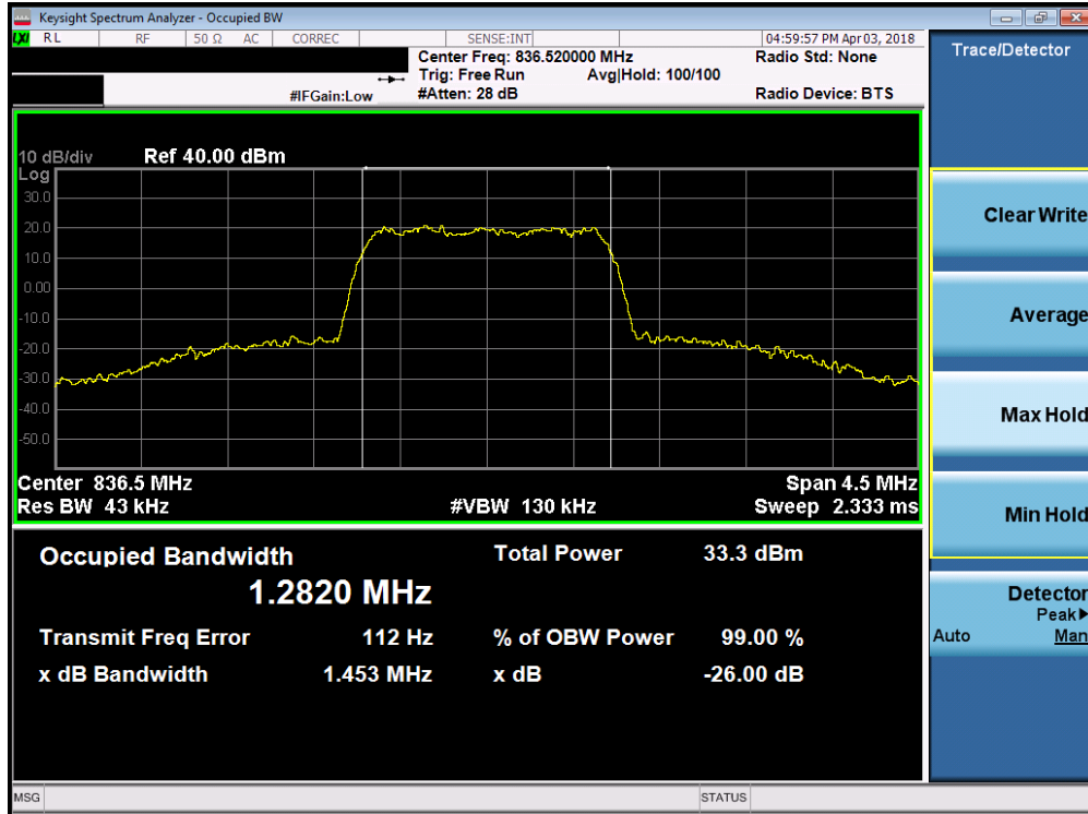
Plot 7-5. Occupied Bandwidth Plot (Cellular CDMA Mode)
