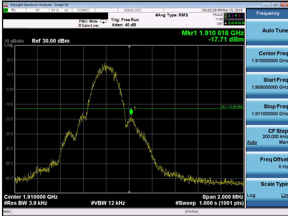
Plot 7-77. Band Edge Plot (PCS GPRS Mode - High Channel)
