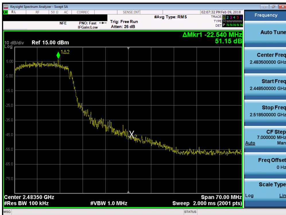
Plot 7-22. Band Edge Plot (802.11g – Ch. 11)
