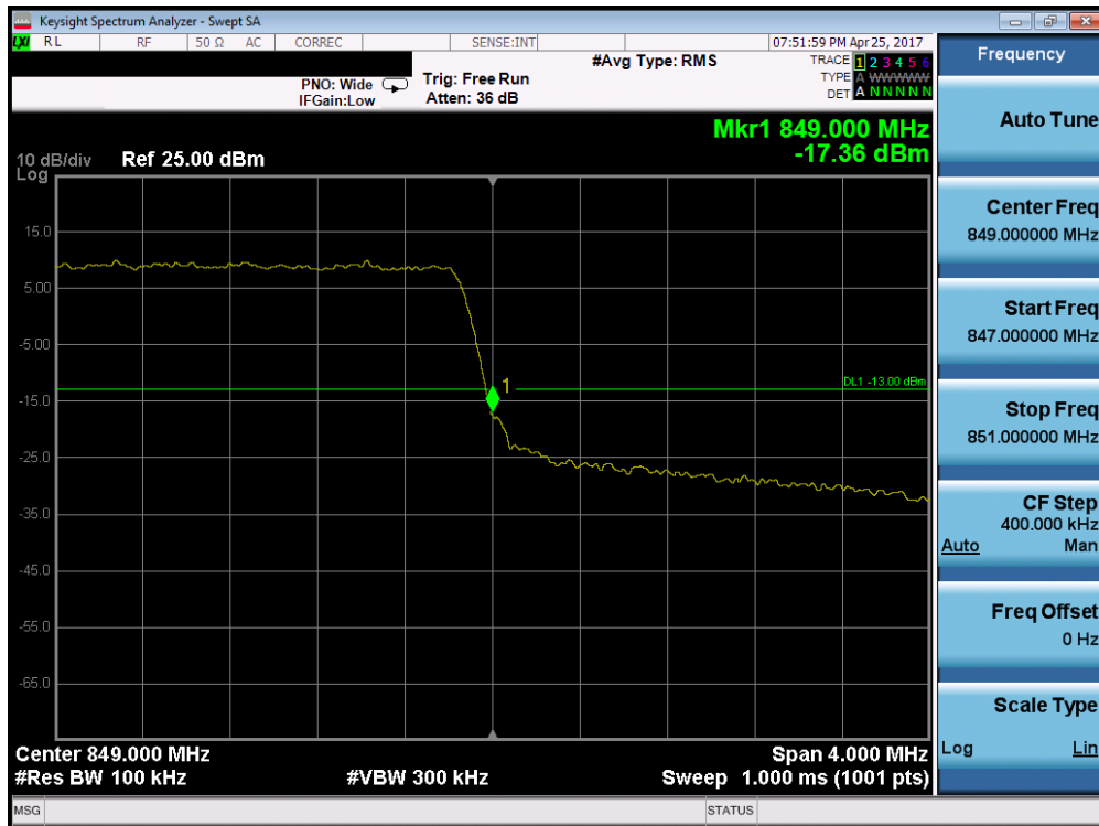
Plot 7-82. Upper Band Edge Plot (Band 5 – 3.0MHz QPSK – RB Size 15)
