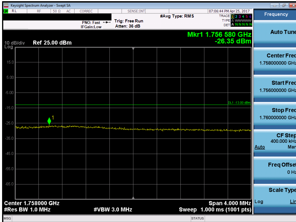
Plot 7-106. Upper Extended Band Edge Plot (Band 4 – 15.0MHz QPSK – RB Size 75)
