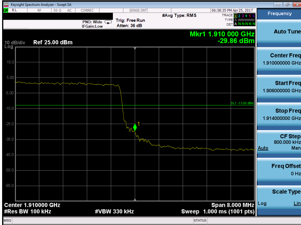
Plot 7-125. Upper Band Edge Plot (Band 2 – 10.0MHz QPSK – RB Size 50)
