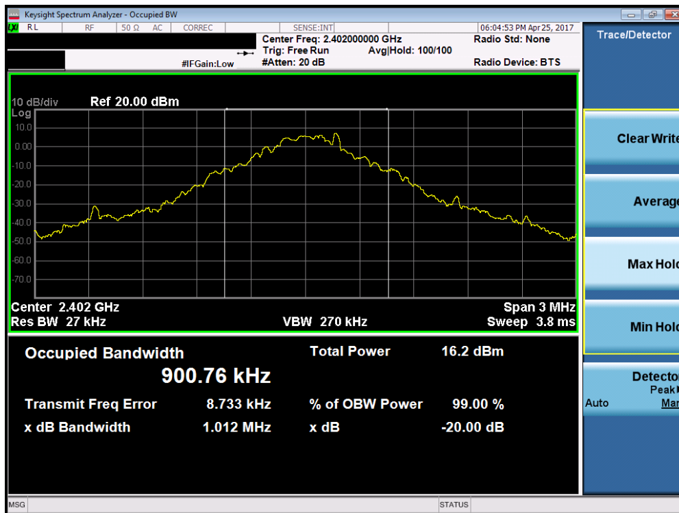
Plot 7-1. 20dB Bandwidth Plot (Bluetooth, 1Mbps – Ch. 0)
