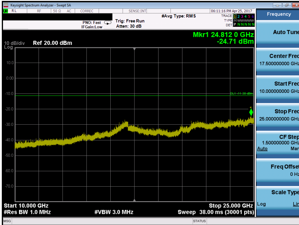
Plot 7-41. Conducted Spurious Plot (Bluetooth, 3Mbps – Ch. 78)
