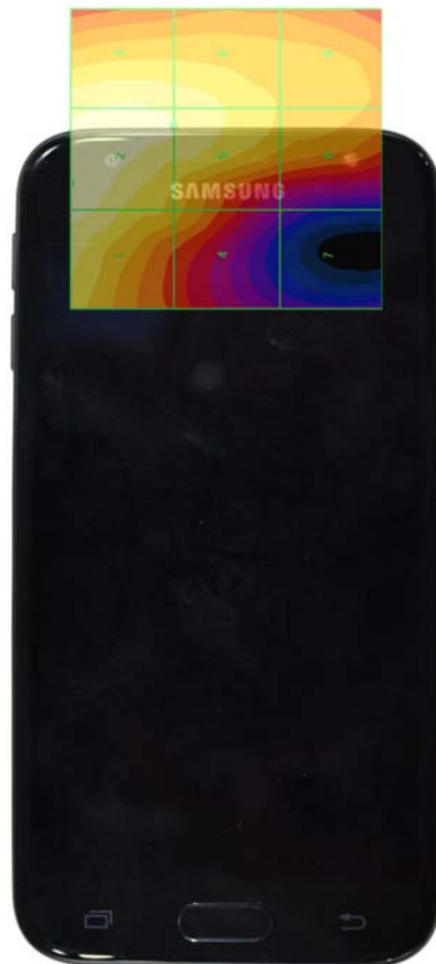
Figure 17-4 E-Field WD Scan overlay
