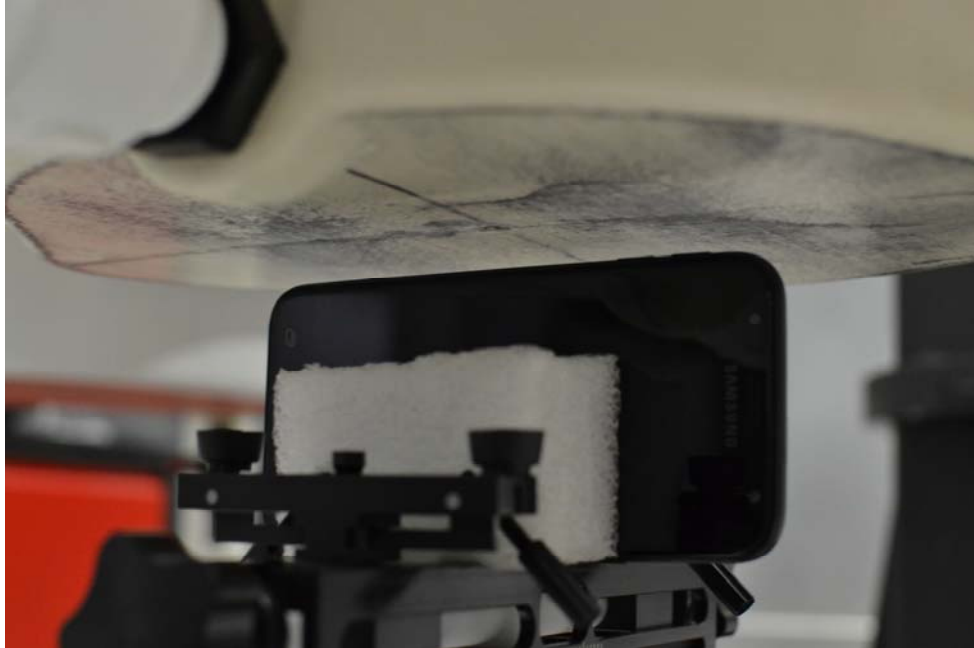
SAR Test Setup Photo 11 – Left Edge at 10 mm
