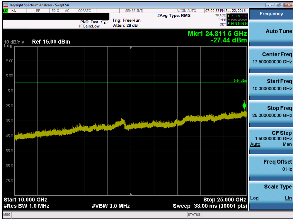
Plot 7-39. Conducted Spurious Plot (Bluetooth, 3Mbps – Ch. 39)
