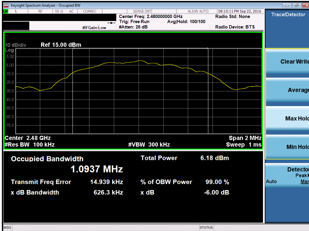
Plot 7-3. 6dB Bandwidth Plot (Bluetooth (LE) – Ch. 39)
