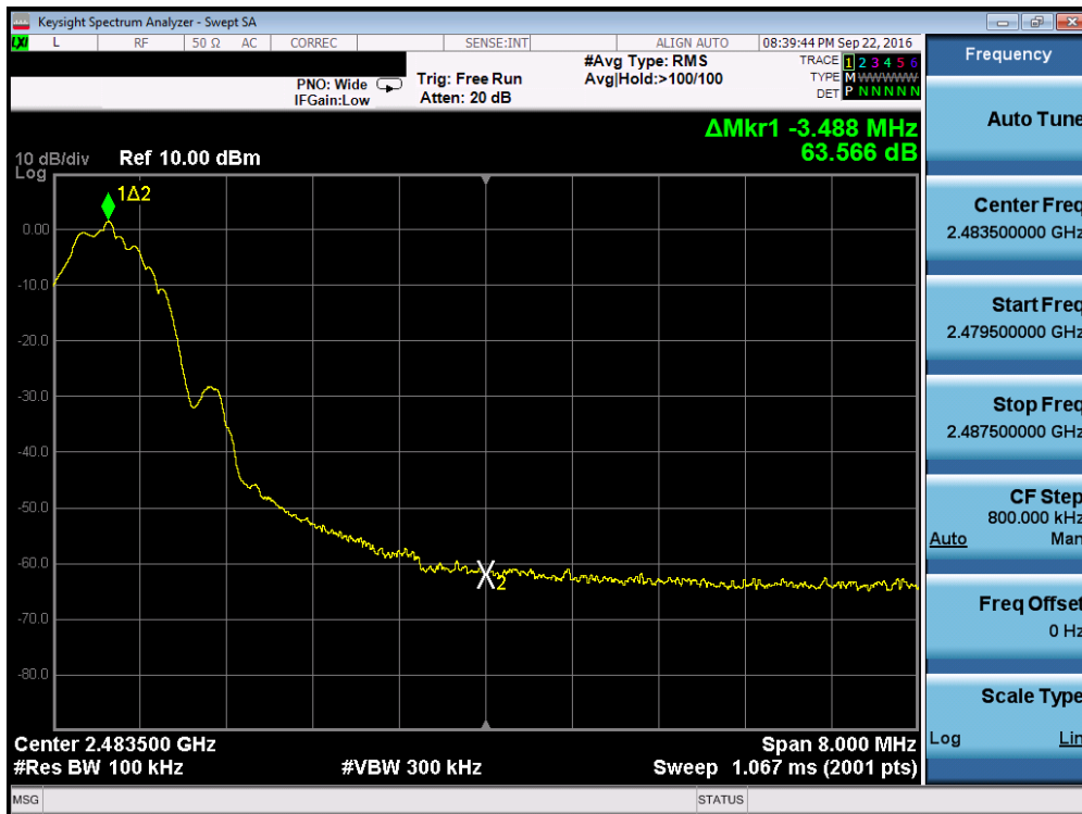
Plot 7-11. Band Edge Plot (Bluetooth (LE) – Ch. 39)
