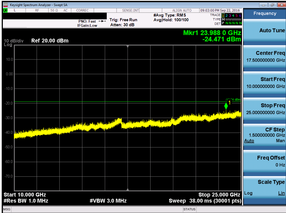
Plot 7-15. Conducted Spurious Plot (Bluetooth (LE) – Ch. 19)
