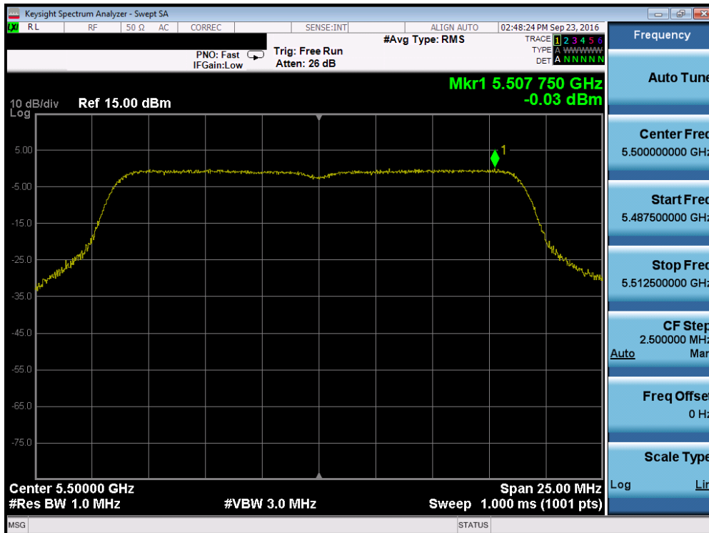
Plot 7-53. Power Spectral Density Plot (20MHz BW 802.11n (UNII Band 2C) – Ch. 100)
