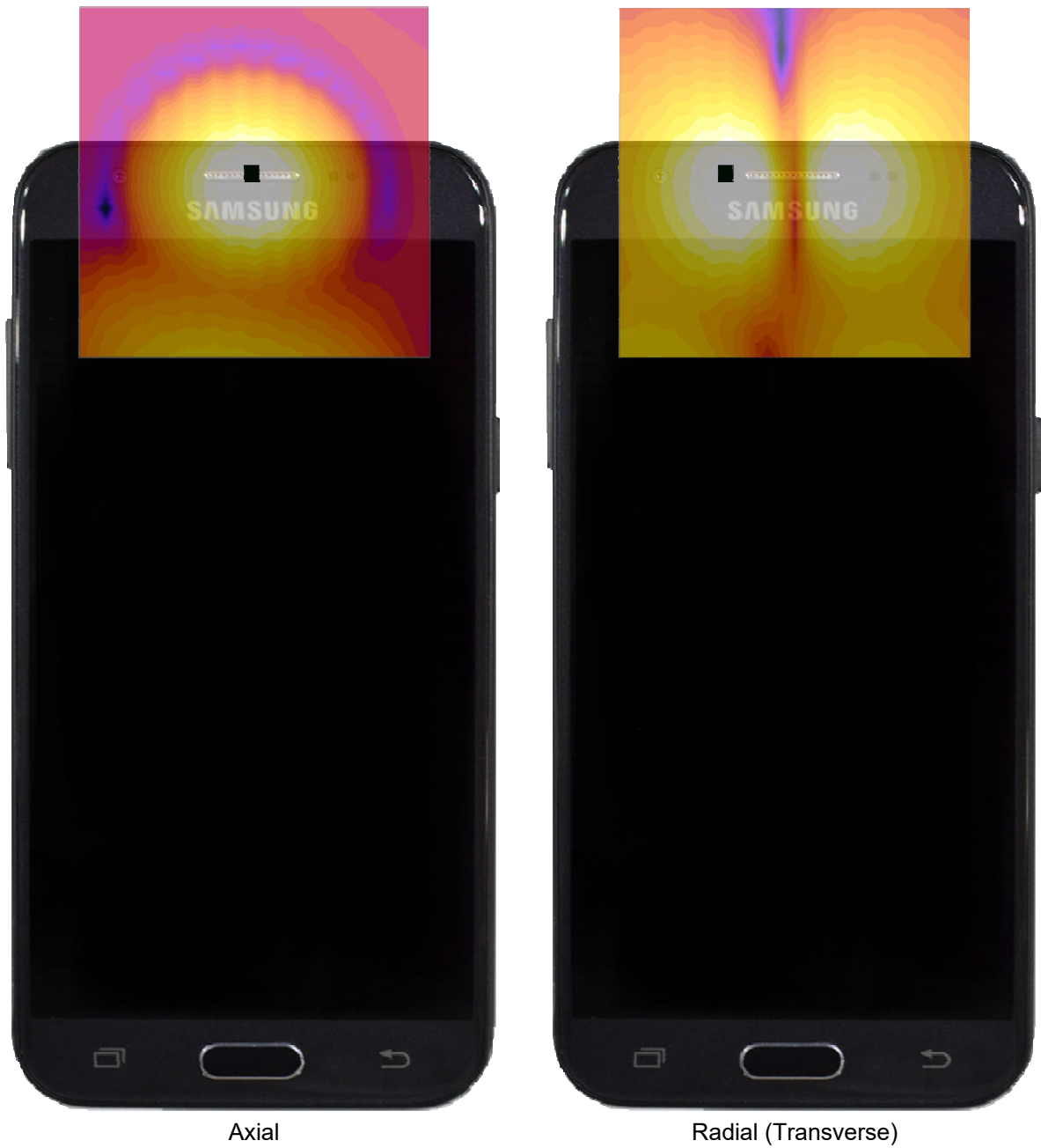
Figure 14-3 T-Coil Scan Overlay Magnetic Field Distributions
